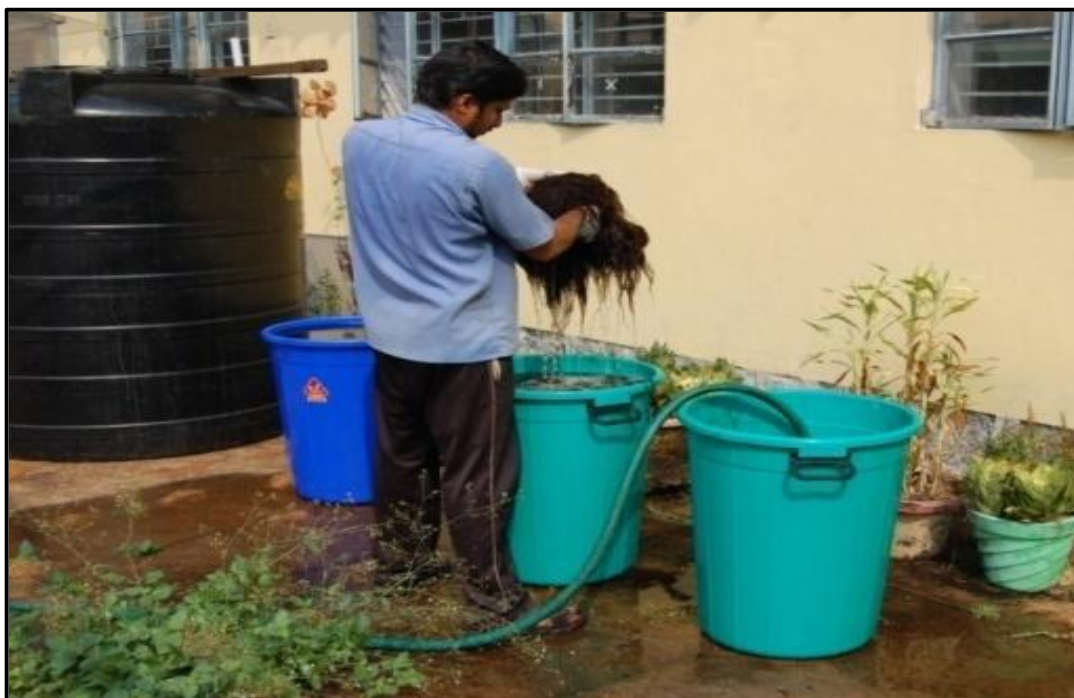
Fig. 12 Alkaline permanganate treatment of FT-03
