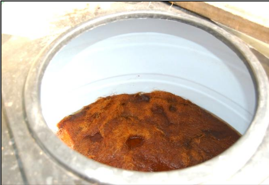
Fig. 4 Alkali treated fibre
