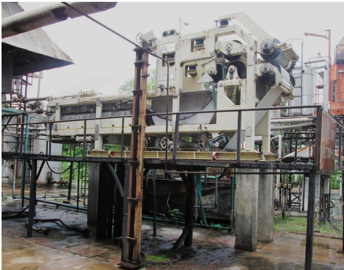
Fig. 27 A view of the double belt washer employed for washing cooked pulp obtained from pilot plant experiment
