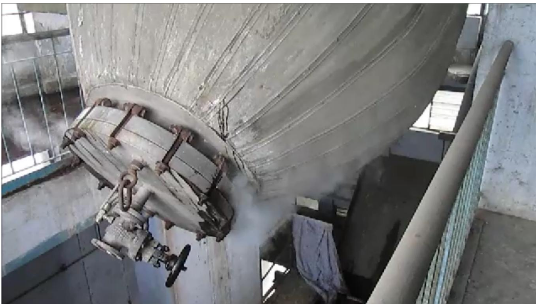
Fig. 25 Digestion of FT-03 in Pilot Plant digester in progress
