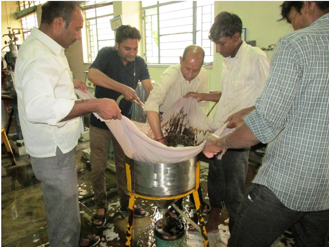
Fig. 30 Final washing of unbleached pulp by manual process
