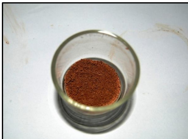
Fig. 6 (b) Precipitated lignin obtained from liquor
