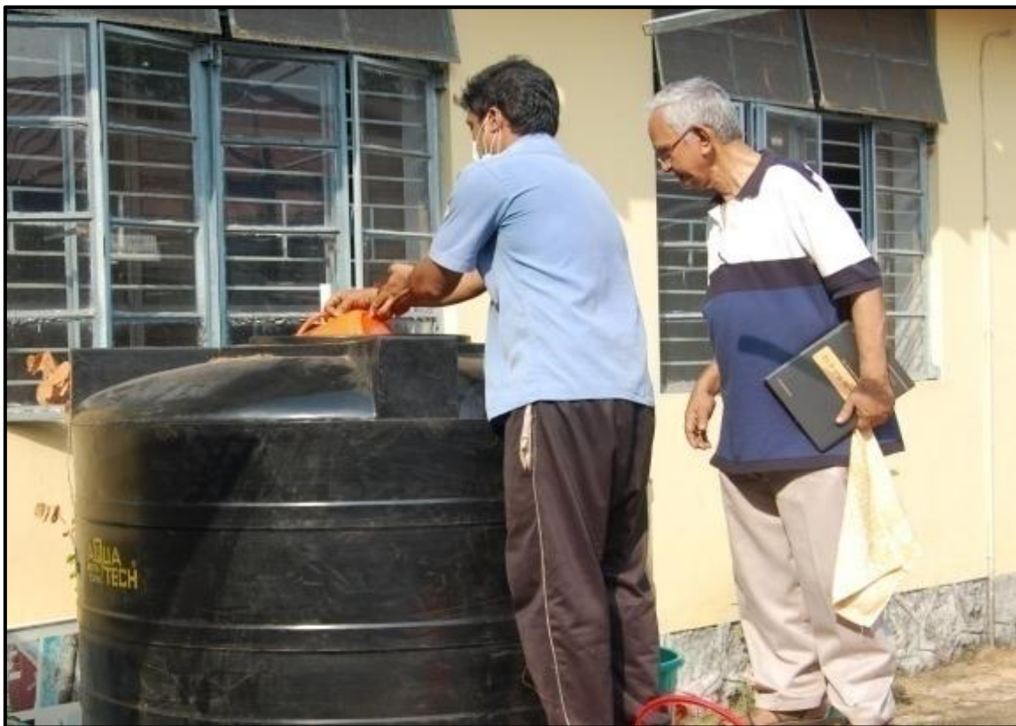
Fig. 2 (b) Application of urea solution on the coconut husk in reaction tank
