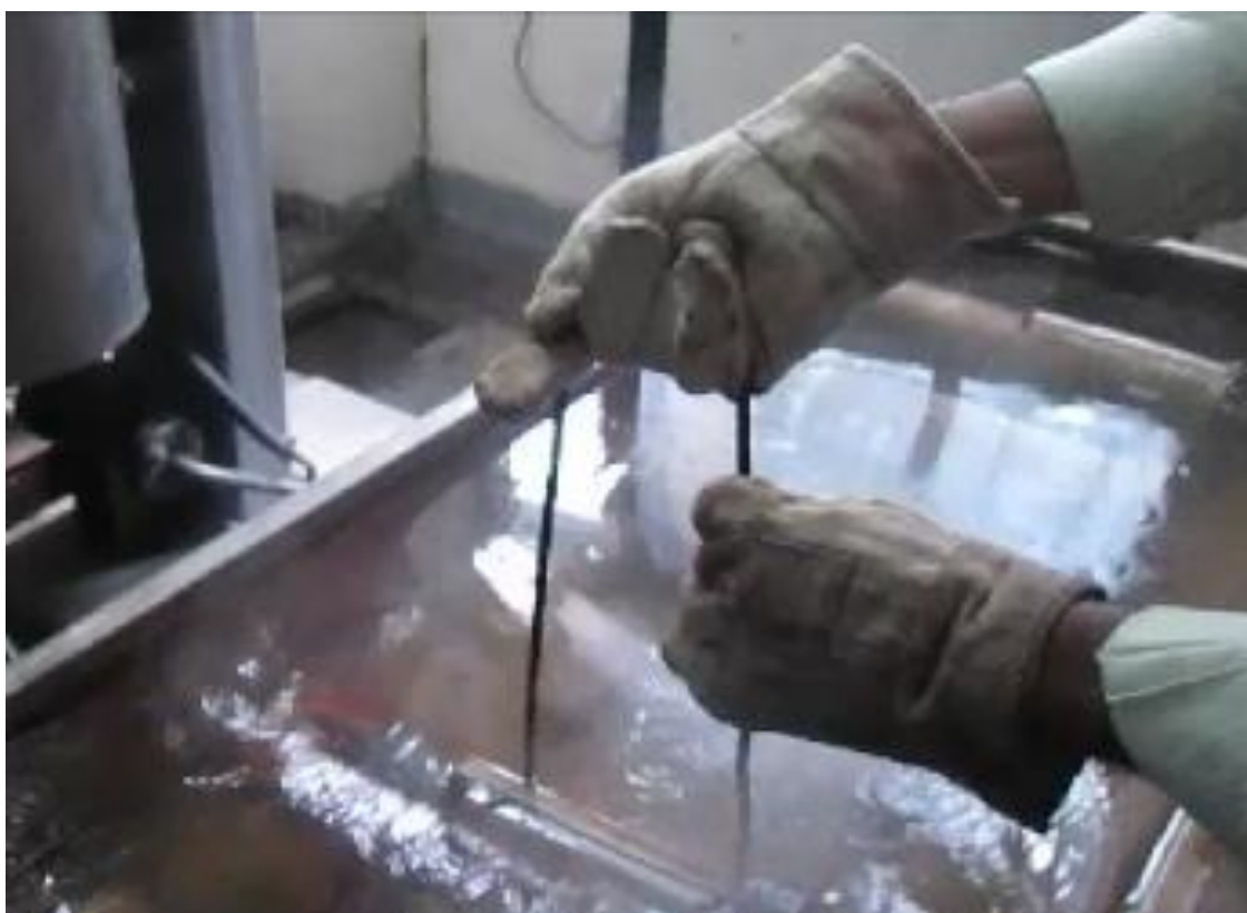
Fig. 17 A bomb being taken out from digester chamber after the cooking is over (top) and immediately dipped in a water tank to stop the reaction (bottom).
