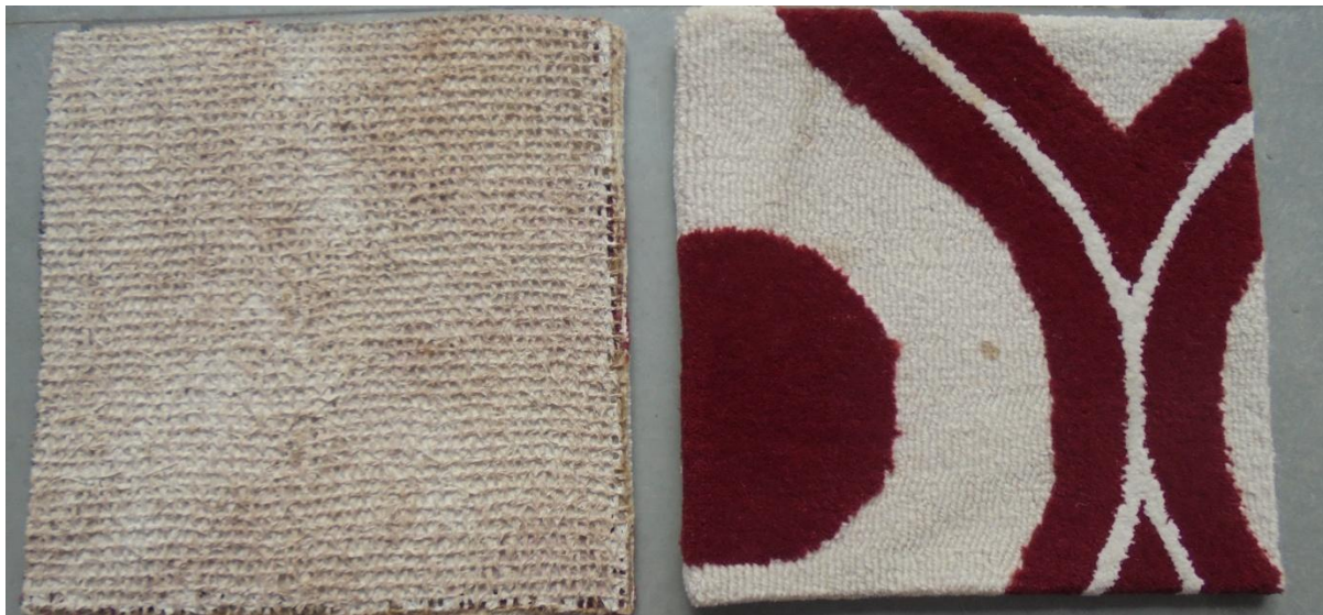
Fig. 45 Carpet backing produced with high density coir scrim fabric; (A) Back side and (B) front side of woolen carpet
