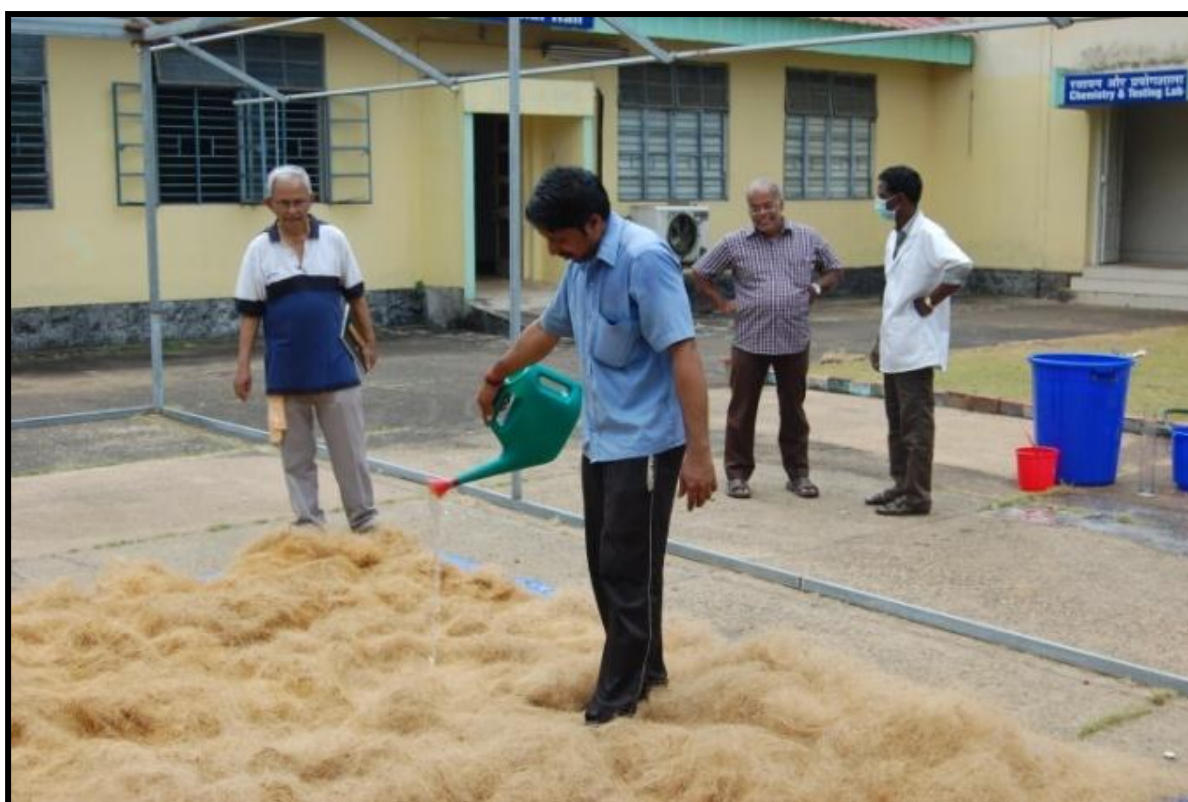
Fig. 1 (b) Application of urea solution to raw coconut husk by hand spray technique
