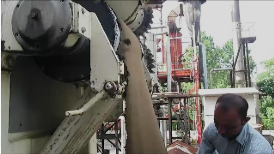
Fig. 28 Pulp sheets being collected after primary washing in the double belt washer
