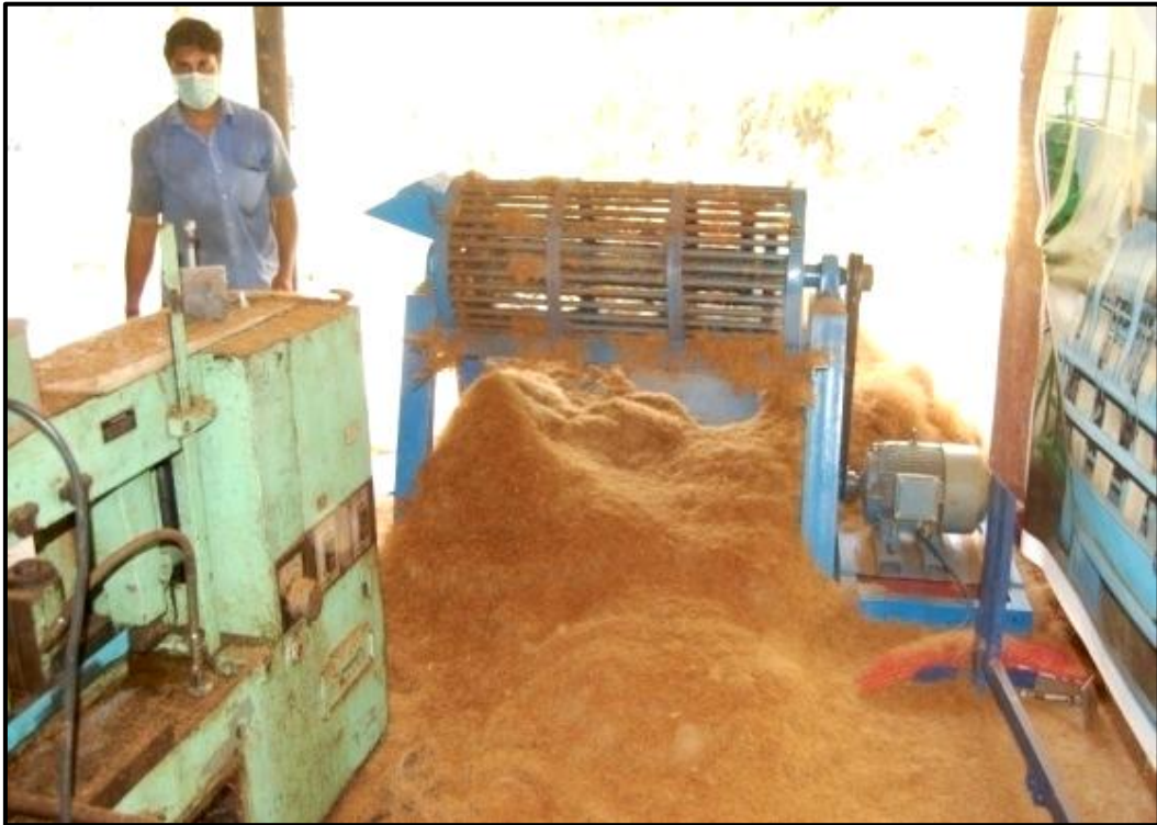
Fig. 13 Bit fibres generated during willowing operation.
