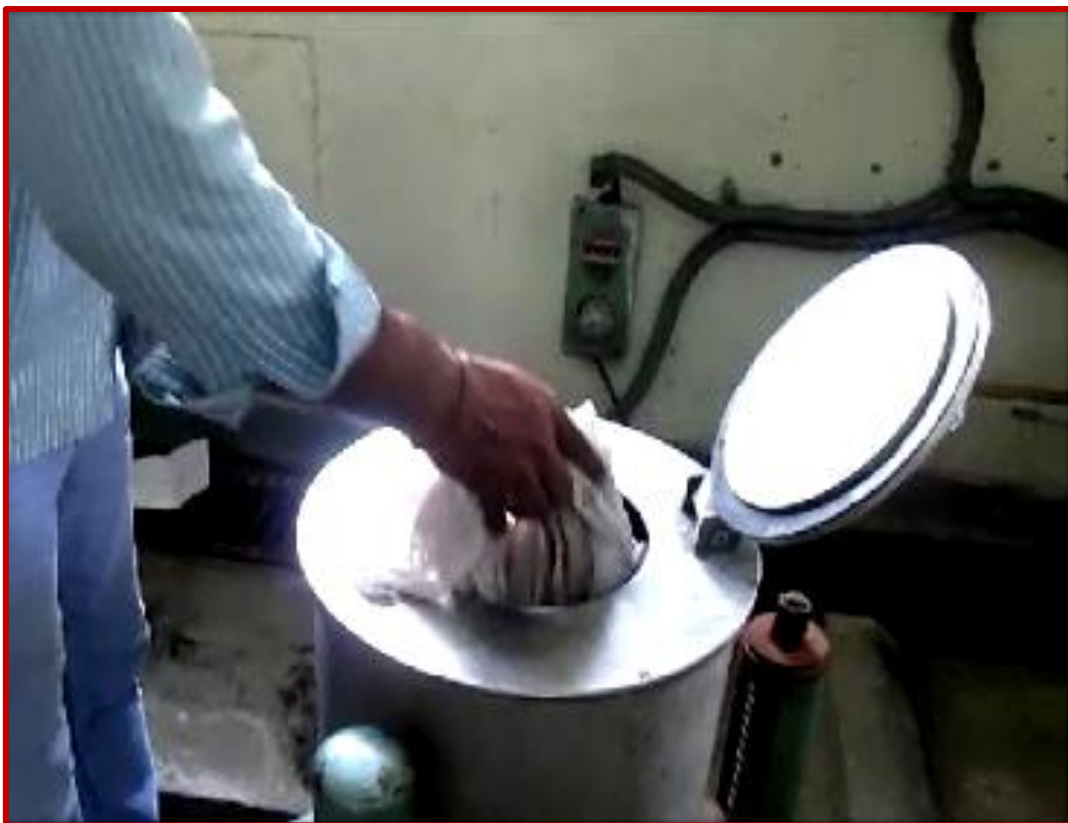
Fig. 19 Hydroextraction of cooked pulp
