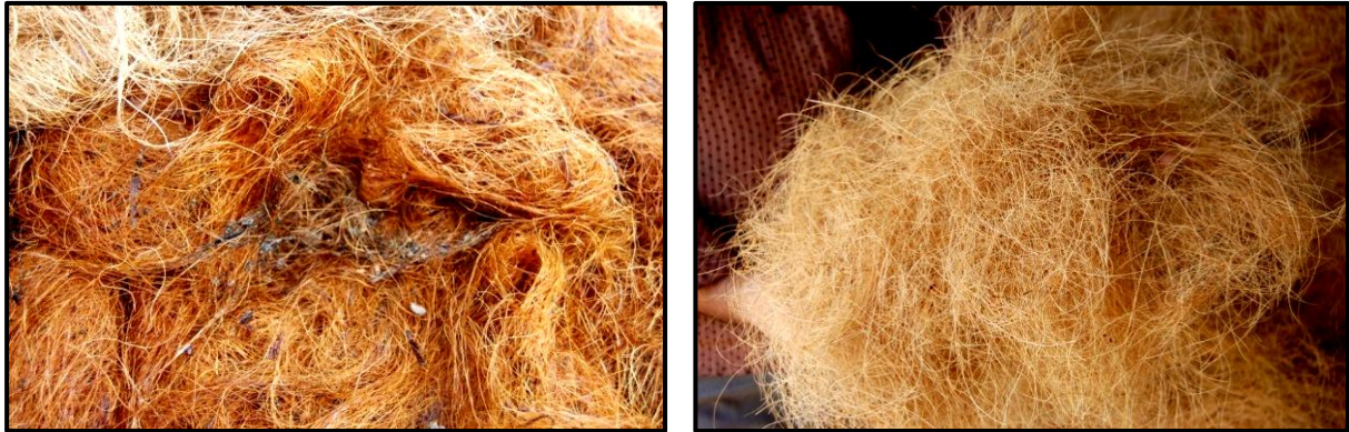
Fig. 11 Alkali extracted fibre before (left) and after (right) willowing. The removal of pith and other impurities is clearly visible.
