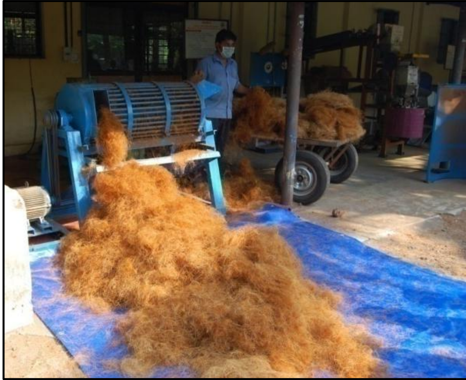
Fig. 9 Willowing in 'Swarna' – a heavy duty fibre extraction machine
