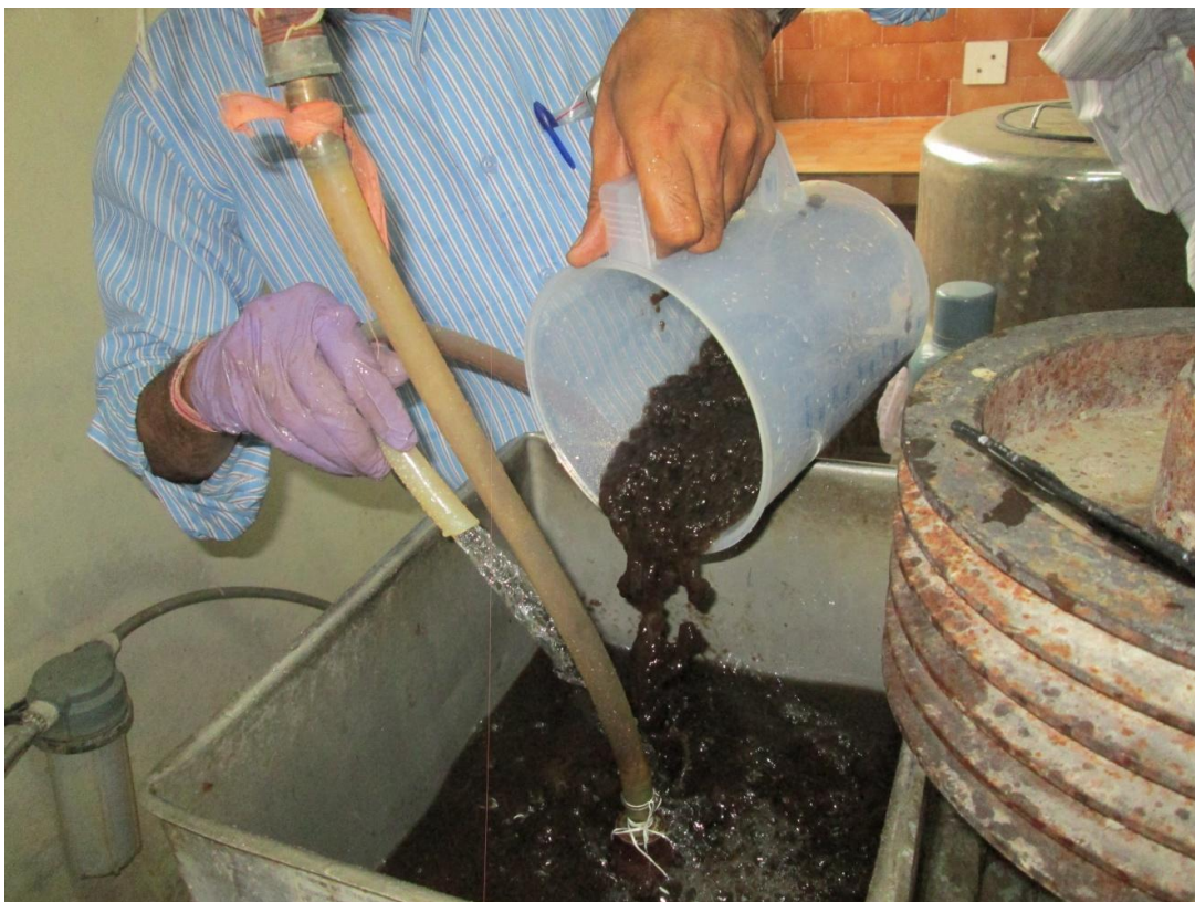
Fig. 31 Separation of rejects by passing through 0.2 mm screen.
