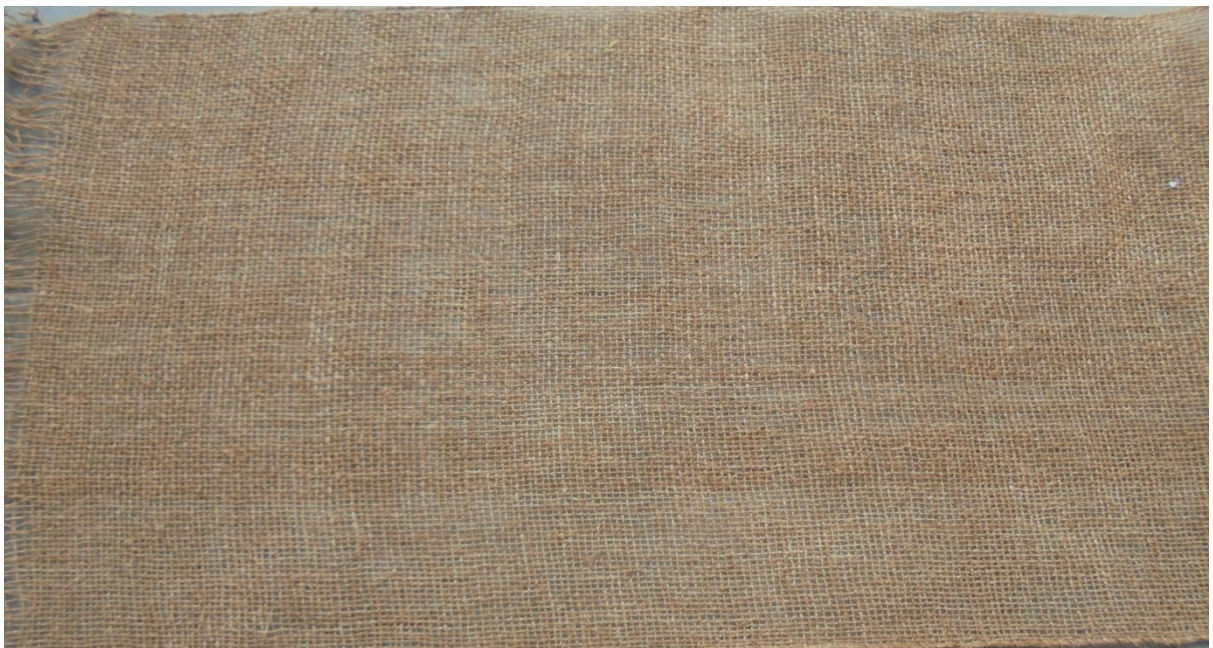
Fig. 41 Coir scrim fabric made from 2- ply coir-sisal blended yarn (80:20%)
