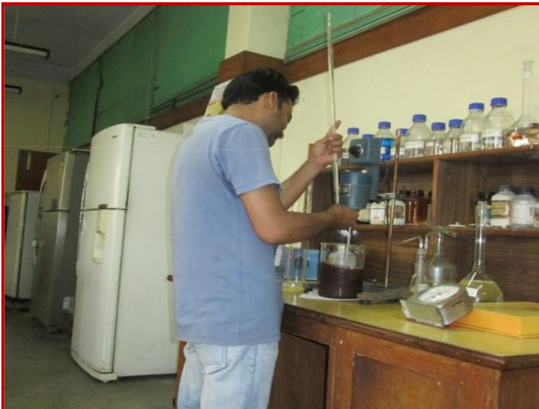
Fig. 21 Determination of kappa number using screened pulp
