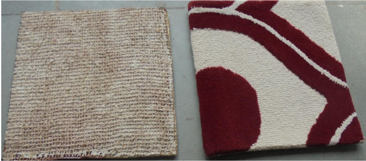
Fig. 44 Carpet backing produced with high density coir scrim fabric; (A) Back side and (B) front side of woolen carpet
